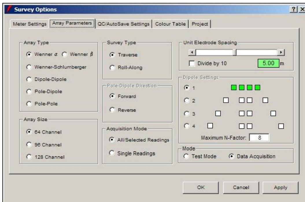
**Figure 4:** The Array Parameters tab
