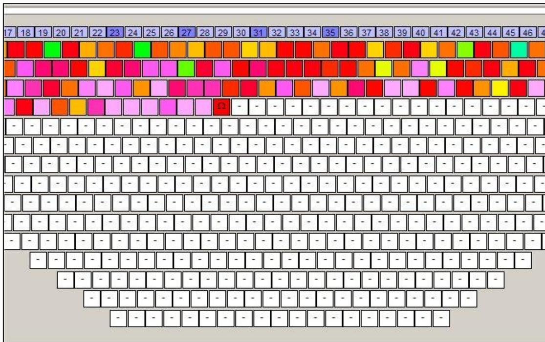
**Figure 9:** Display of data in the Survey Designer pseudo-section display during data collection.
