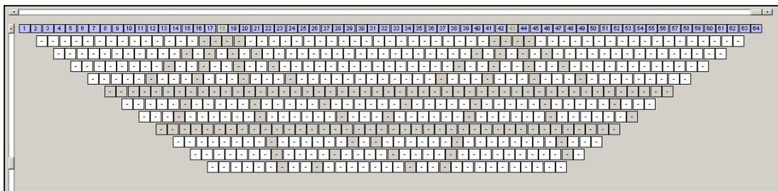
**Figure 2:** Deselected electrodes and their associated measurement positions are greyed out in the Survey Designer window. Individual measurements can also be toggled on / off (see Section 3.6)
