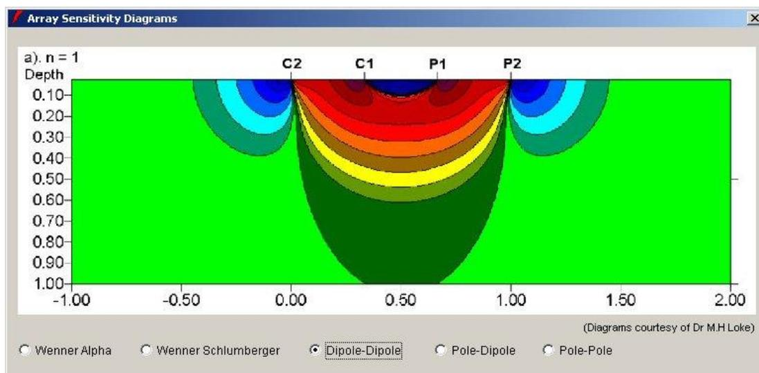
**Figure 15:** Array Sensitivity Diagram selection window
