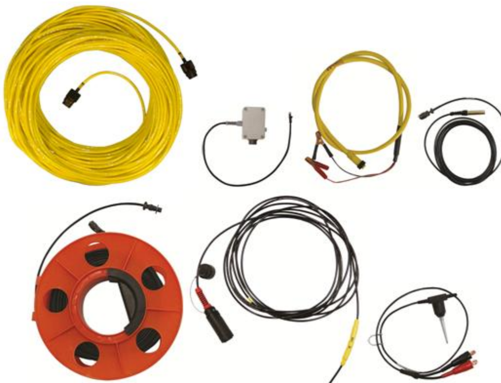
Figure B-3: Typical Geode accessories, clockwise from upper-left: digital interface cable, network interface box (NIB), power cable, hammer switch, trigger extension cable, geophone cable, geophone.
