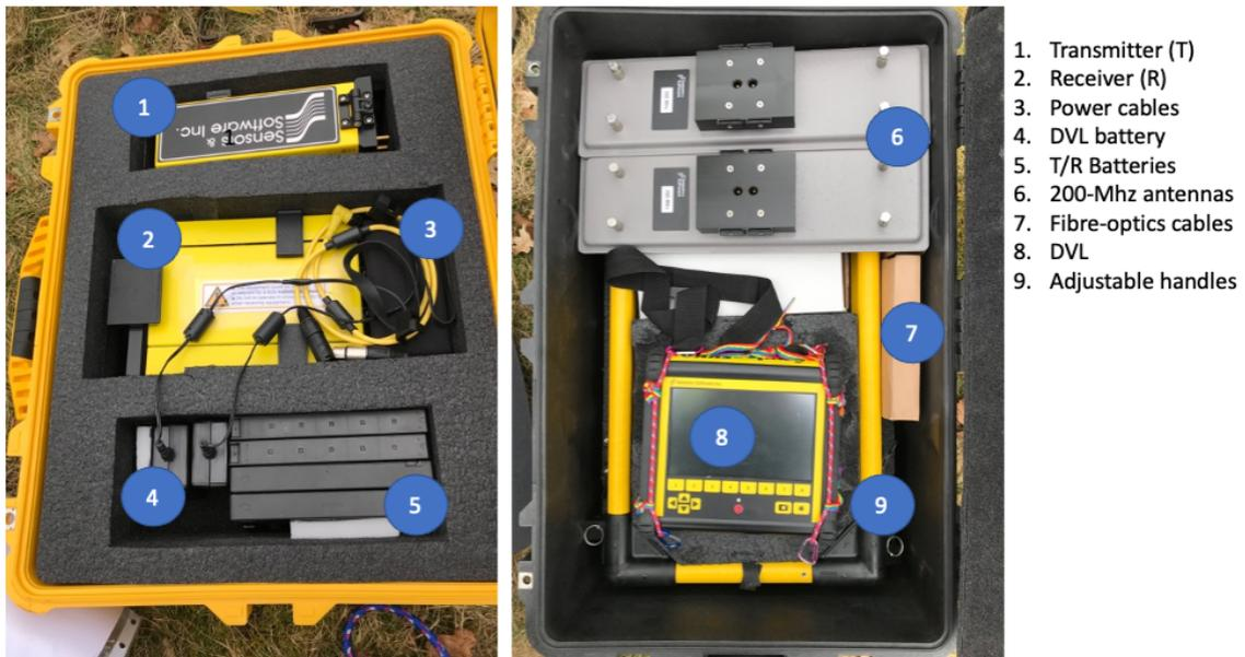
1) Layout of the GPR equipment in the two storage boxes
