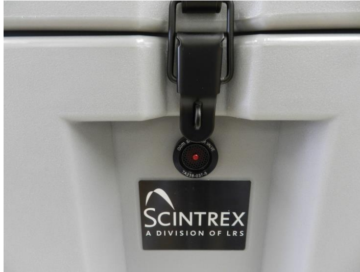
Figure 2-2 Location of the pressure release valve on the transportation case
